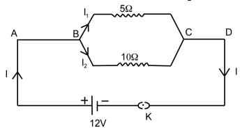
In the given circuit diagram calculate the current  $I_2$  through the resistor of  $10\Omega$ .
